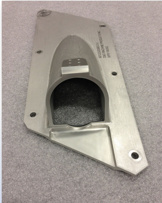
Aerospace – Precision machining from solid aluminum block Nitrogen retro fairing relief valves – Delta Rocket
